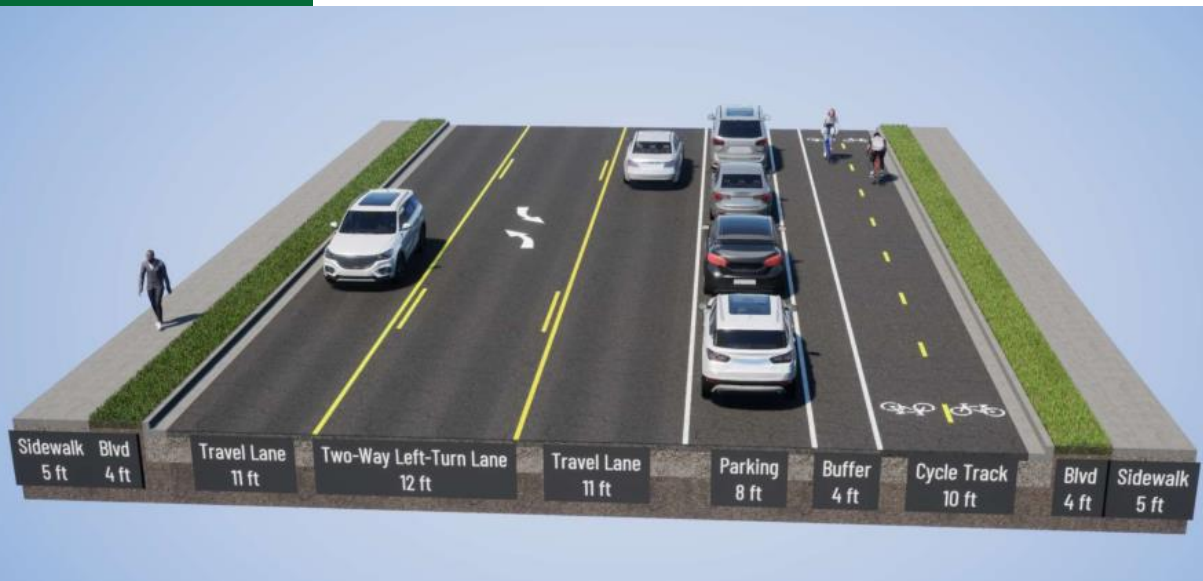
3-Lane Section: 2-Way Cycle Track, Parking 1 side
