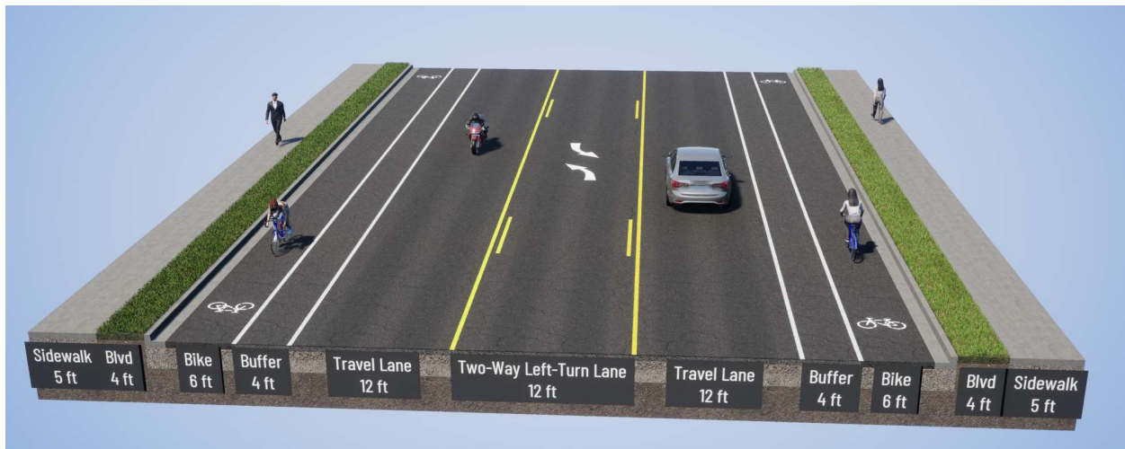
Figure 6 – 3-lanes with buffered bike lanes
