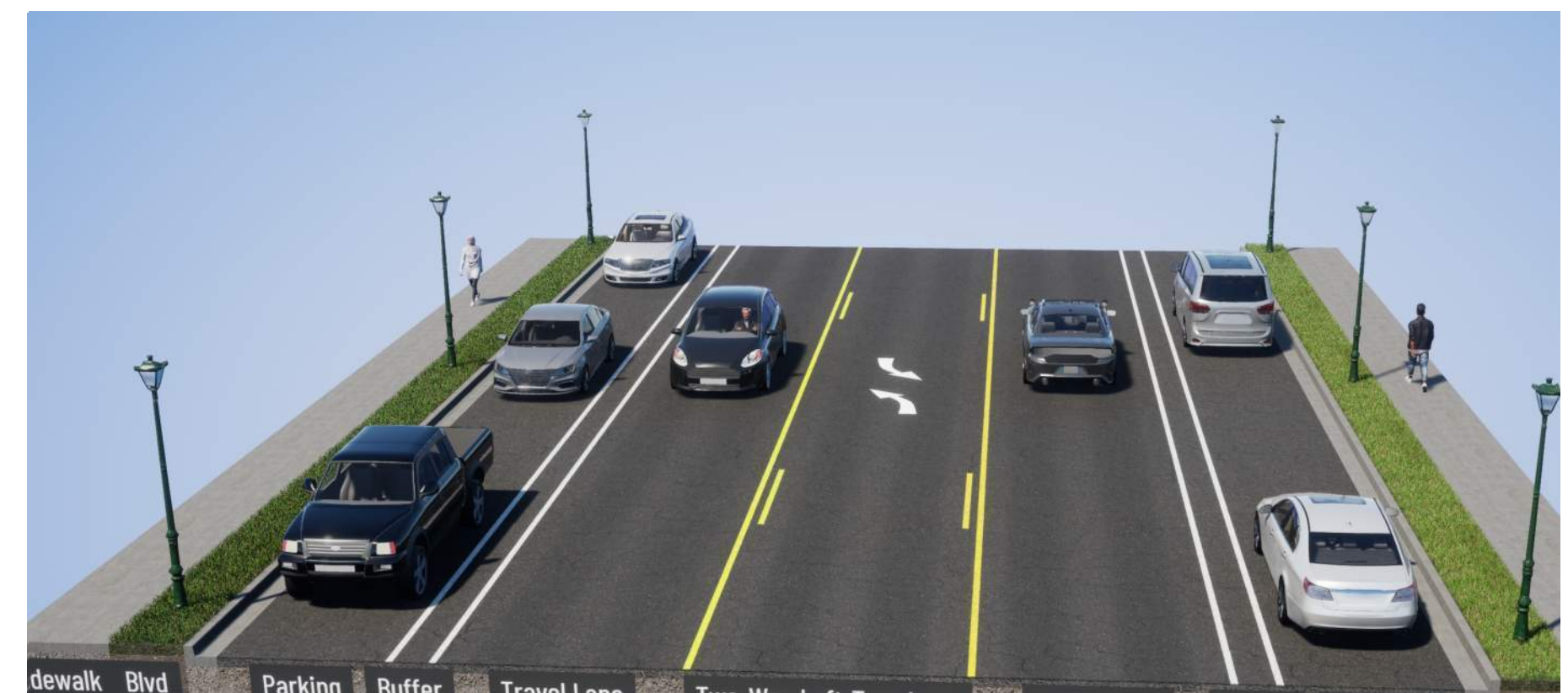
4 TWO-WAY LEFT TURN LANE 5 ft 4 ft 8 ft 2 ft 12 ft 12 ft 12 ft 2 ft 8 ft 4 ft 5 ft sidewalk Blvd Parking Buffer Travel Lane Two-Way Left-Turn Lane Travel Lane Buffer Parking Blvd sidewalk
